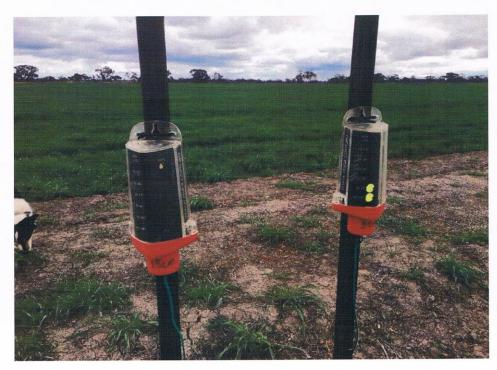
Unfortunately the data wouldn't download off the **Irrometer with the Gypsum Blocks**, however this has proven to be reliable moisture meter that can either be read in the paddock or downloaded on a data logger and viewed in a graph on a computer.
